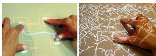
Figure 3: Examples of uses a multiple pointing input: left: curve editing. right: a map browsing system. The user can use one finger for panning, or two fingers for simultaneous panning and rotating
