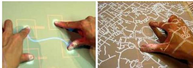
Figure 3: Examples of uses a multiple pointing input: left: curve editing. right: a map browsing system. The user can use one finger for panning, or two fingers for simultaneous panning and rotating
